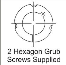
Keyways are British Standard Imperial B.S. : 10 : Part 1:1972 and conform to I.S.O. recommendations except for the bore sizes marked\* which are shallower. Where a key is to be used it should be parallel and side fitting with top clearance. Depth of keyway is measured at CROWN.
